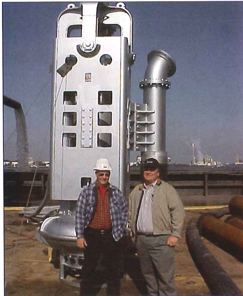
Toyo DP-400-16 in. discharge & weighs 24,000 lbs
